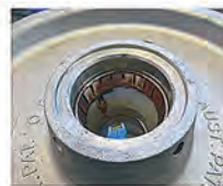
INTEGRAL (15", 16", 18") Image shows area where seal fits
