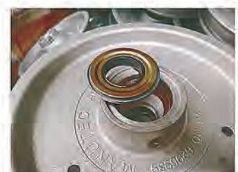
The picture above is the model (pre 2013). It has the recessed area and needs to have the spacer washer (pictured above fitted)
