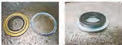
The picture on the left hand side is the new model (post 2013). If you have this model then no washer is required.
